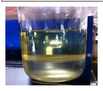
Slops is the fuel drained off to perform samples and quality control tests that cannot be returned
